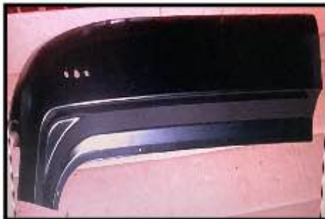
屋頂水槽 左 Roof rail
