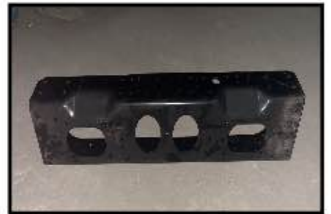
前橫梁 Front reinforcement
