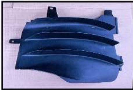
角板通風網 左 Corner panel ventilation base
