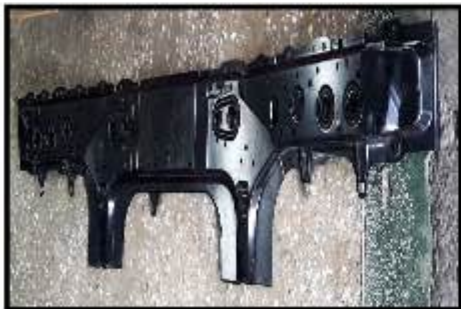
面板加強樑 Panel reinforcement
