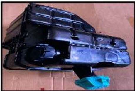
副水桶 Water tank
