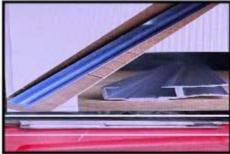
玻璃導槽 Glass channel
