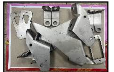
遮陽板 支架/白鐵 Sun visor bracket/stainless steel
