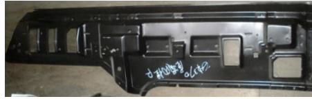
EXR430003 屋頂水槽內裡 左 ROOF SINK INNER LH
