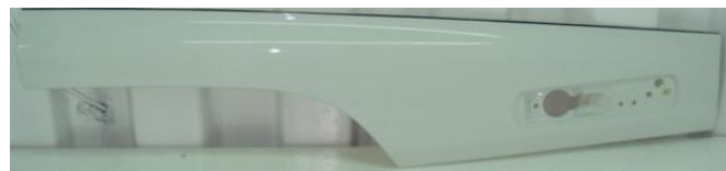
FSR96042 車門外飾板 右下 DOOR OUTER GARNISH BOARD LOWER RH FSR96042A 車門外飾板 右下(電鍍) DOOR OUTER GARNISH BOARD LOWER RH (CHROME)
